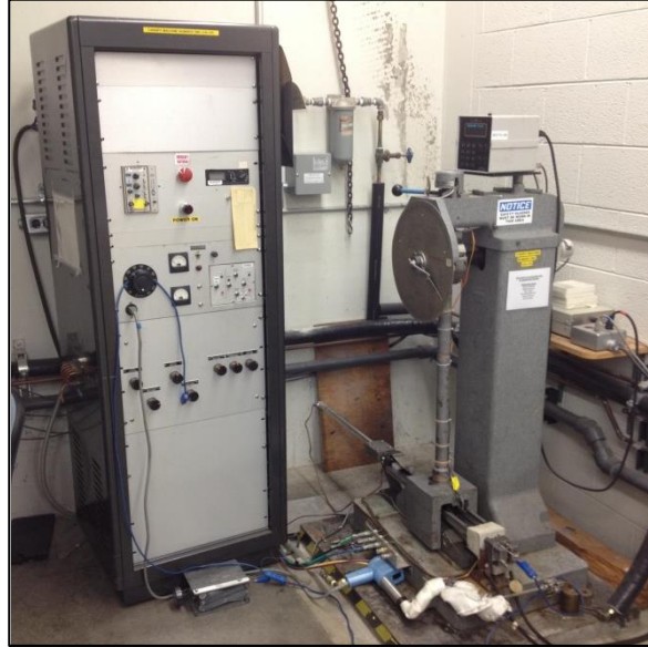
FIG. 1. Views of the Tensile/fracture-toughness testing frame (left) and Charpy impact test frame (right)
