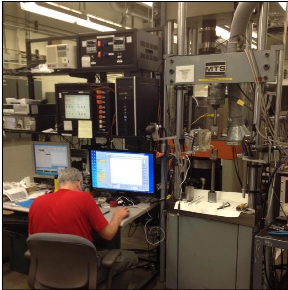
FIG. 1. Views of the Tensile/fracture-toughness testing frame (left) and Charpy impact test frame (right)
