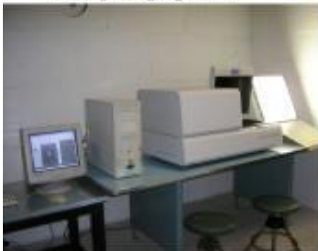
Tomography system with Position Sensitive Detector
