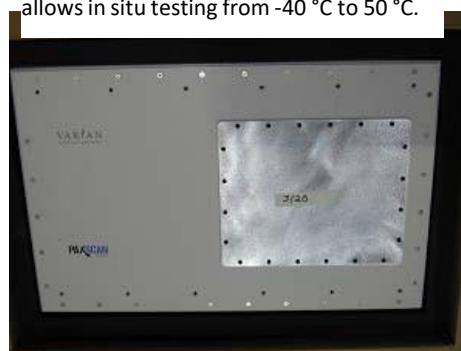
Figure 7. Varian Paxscan detector, 250 μm spatial resolution.
