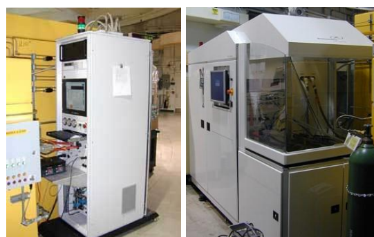
Figure 4. Small Scale fuel cell test stand (left) and industrial scale test stand (right).
