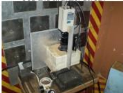
Neutrongraphic system with CCD and cintilator screen
