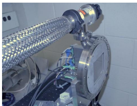
Figure 10. Large microchannel plate detector. FOV 9 cm x 9 cm. Spatial resolution 15 \mu\text{m} .
