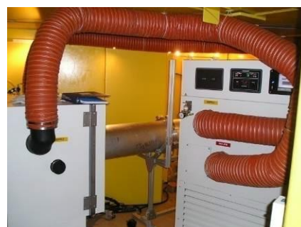
Figure 6. Environmental chamber that allows in situ testing from -40 °C to 50 °C.
