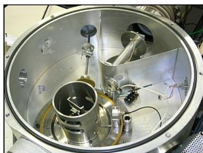
Fig. 1. In-vacuum RBS setup with two detectors and charge shields
