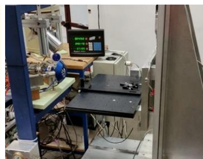
Fig. 3. External beam setup and the robotic table
