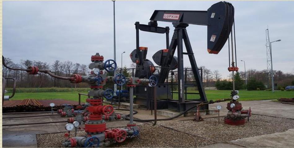
In the case of borehole mining (mainly related to oil and gas extraction) internal surfaces of the installation used and pipelines are often covered with a layer of sediments containing significantly increased concentrations of radium isotopes and Pb-210 and Po-210. The sediments are created from **radionuclides present in formation water** that usually coexists with fossil fuels.
