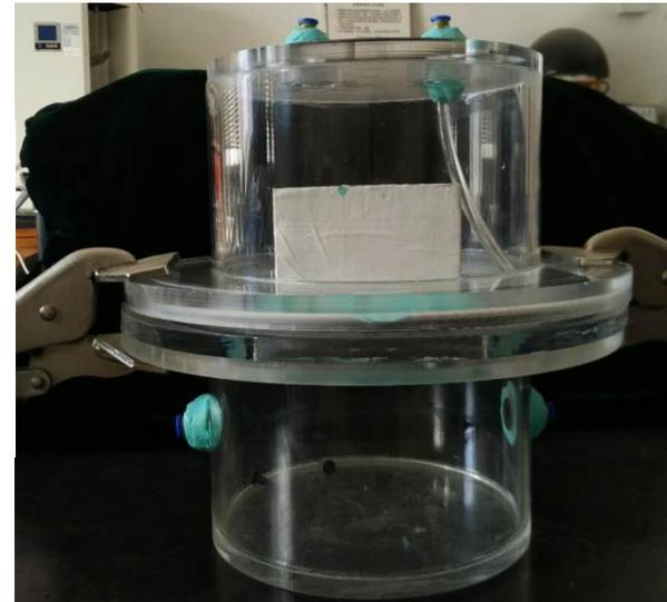
The setup of radon diffusion length measurement
