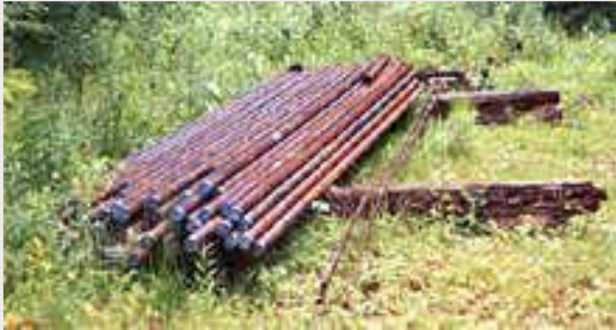
Gas well pipe contaminated with NORM scale, USA
