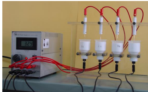
Electrodeposition of radionuclides on discs
