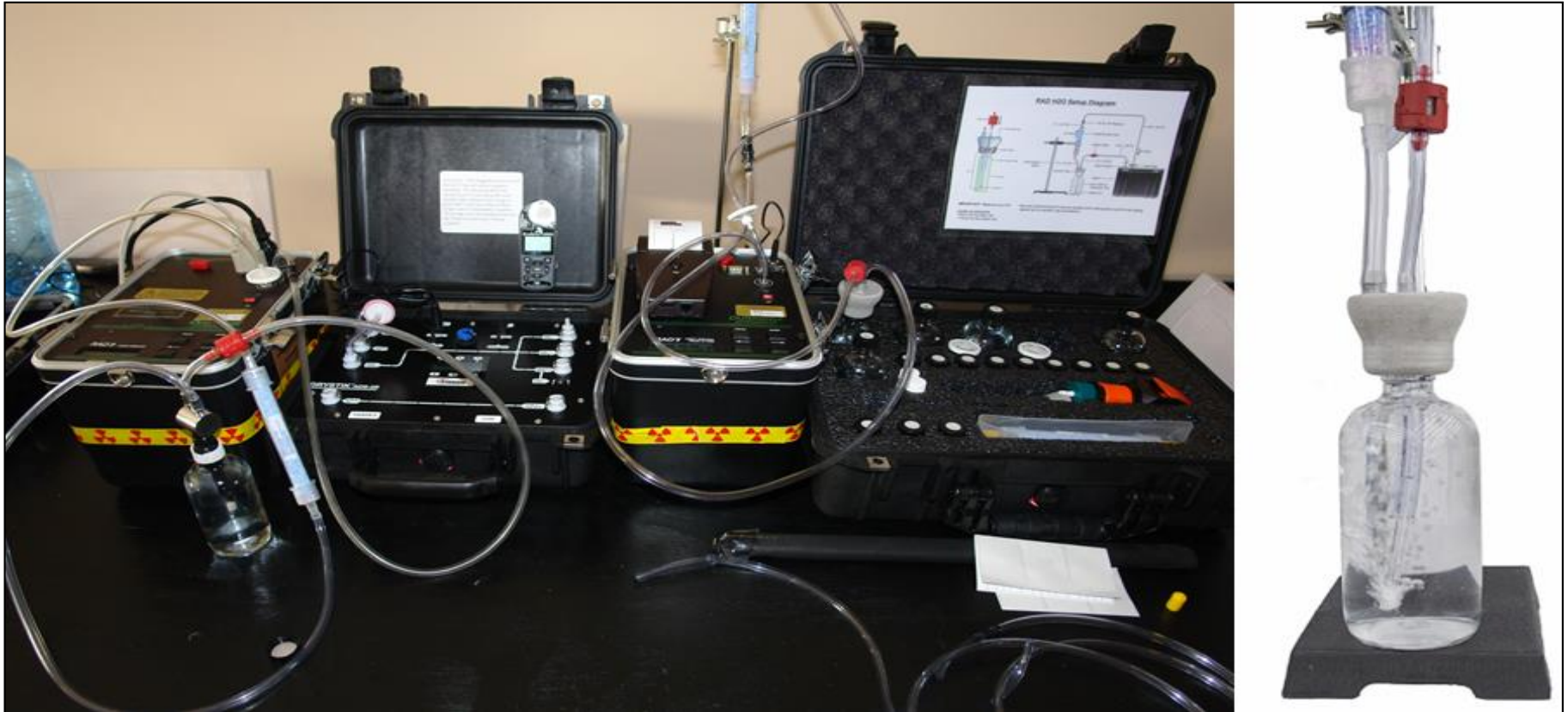
Figure 4: Radon-in-water measurement mobile station making use of two RAD7 detectors, Drystick ADS-3R and H2O kit manufactured by DURRIDGE.
