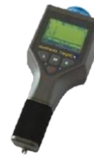
Radionuclide Identifier Device
