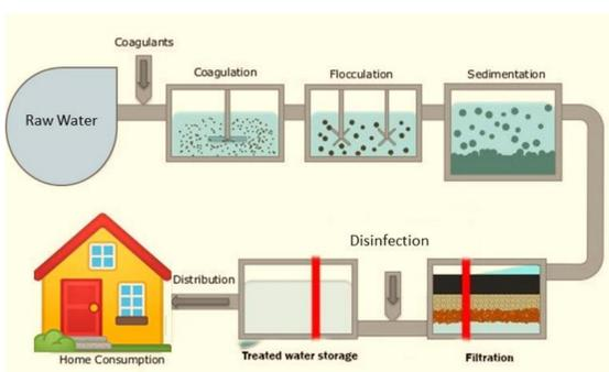
Fig. 1: Generic steps of water purification process [1].
