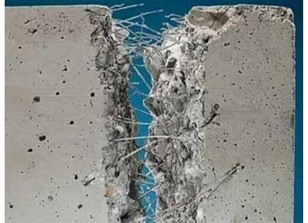
Fig.: fiber-reinforced concrete
