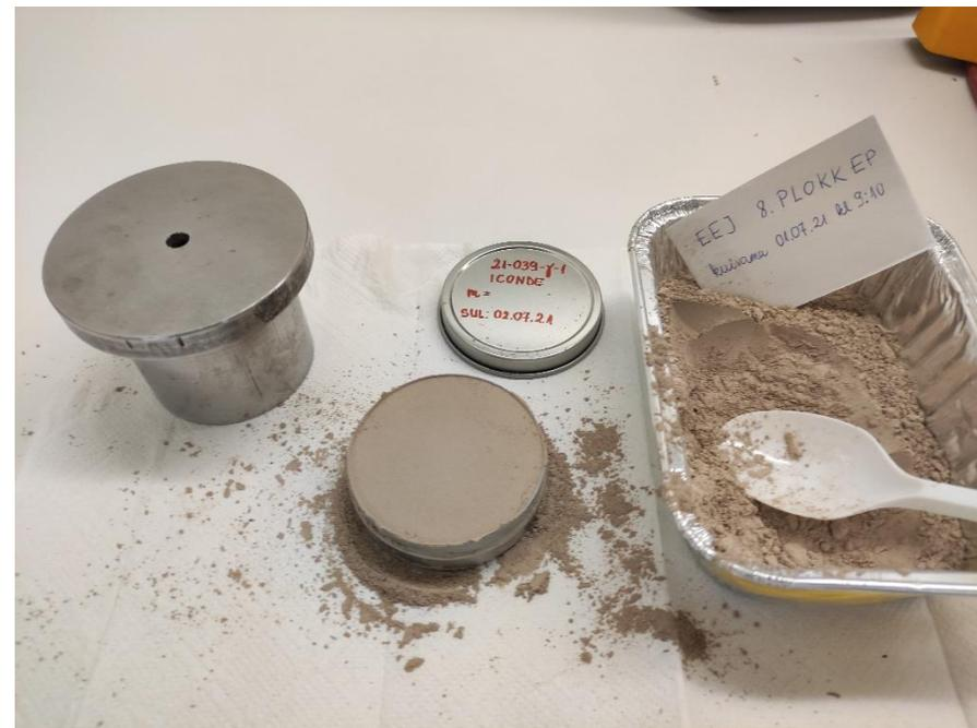
Fig.: Oil shale ash sample
