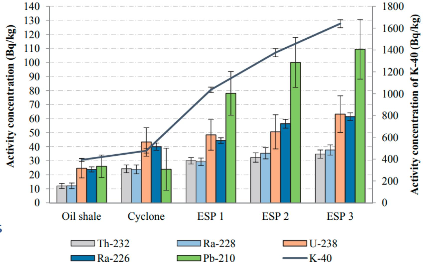
Fig.: Radionuclide activity concentrations (Bq/kg) in different ash fractions of a pulverized fuel boiler (Vaasma, 2017. PhD thesis. University of Tartu). 5(16)
