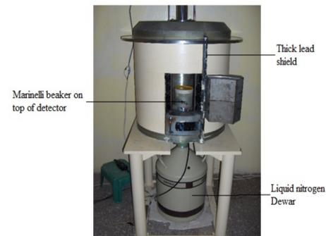
Fig. 2: Radioactivity measurement using HPGe detector
