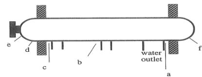
Fig.3: TE-NORM measuring points in a typical FWKO vessel
