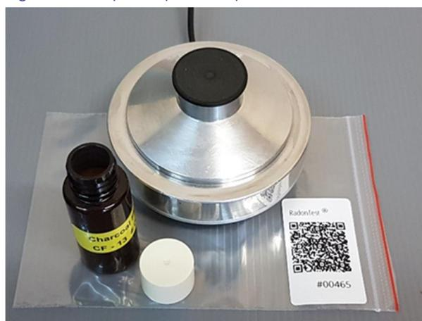
**Equipment for measuring indoor radon using the charcoal method consisting of the detector type BDB-13 and set of samples (usually 20-40), each of which includes the type CF-13 charcoal flacon and the package labeled with the QR-code. The volume of the bottle (charcoal) is 20 (13) mL.**
