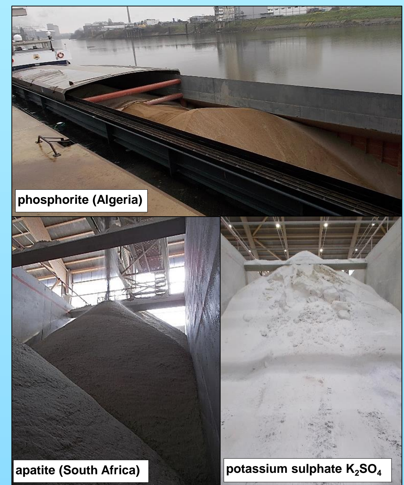
Mass-related activity of different material samples, taken of raw materials, filter dust, final products and dust from the bottom Examples of raw materials with high activity
