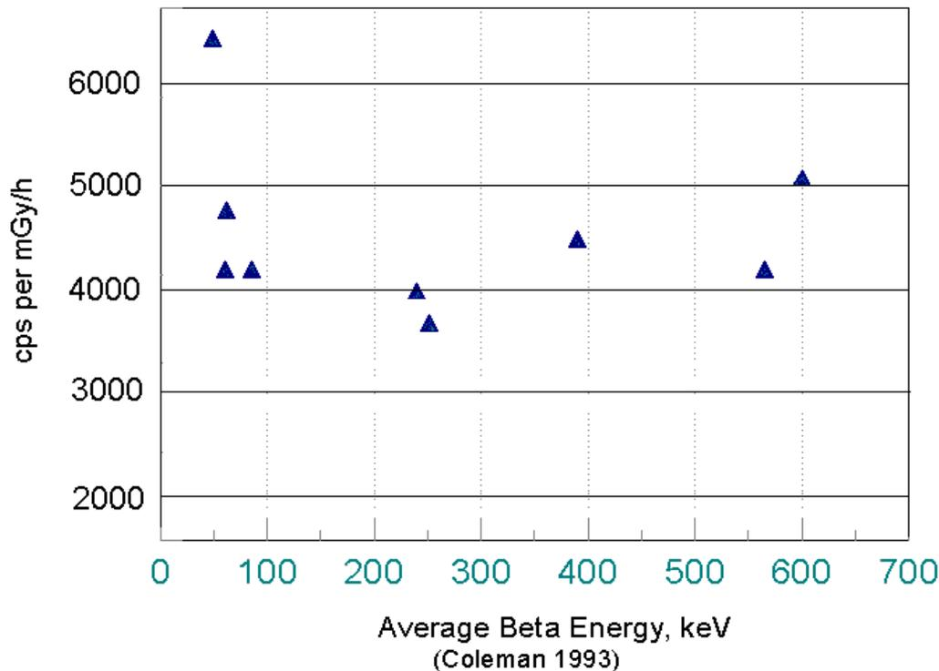
The graph summarizes the expected count rate (counts/minute) per dose rate (mGy/h) as a function of average beta energy for a GM pancake detector with a typical operational configuration.
